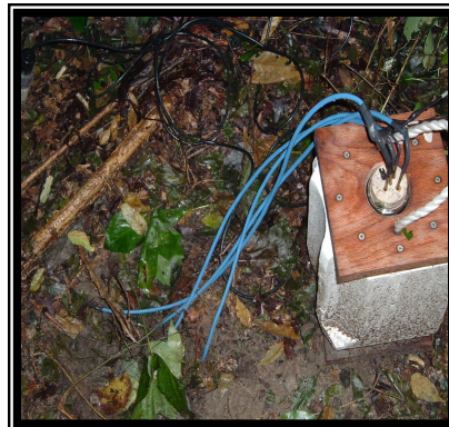
Stable Zero-Point Ice Reference for Thermocouple Temperature Profile Measurements at Four Depths in Soil
