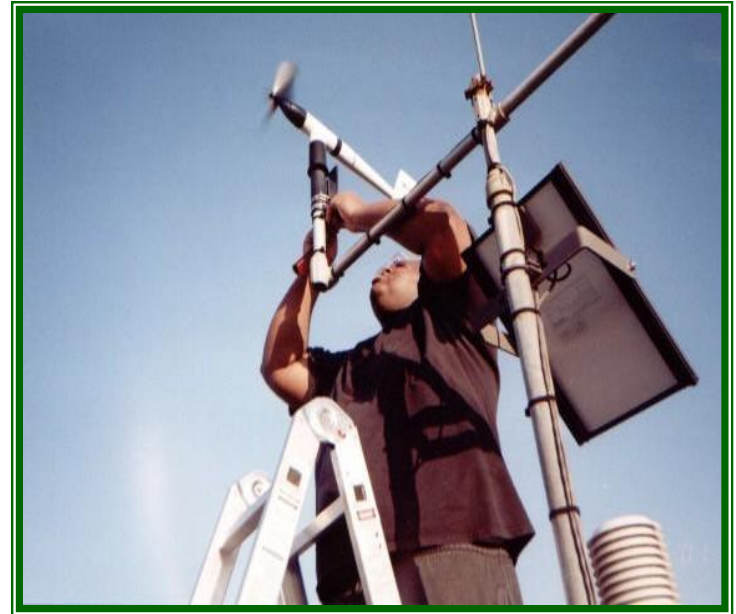
Morehouse College Student Mounting Propeller-Vane Anemometer on Boom
